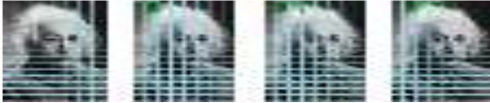
Figure(6): The image is divided into blocks (8x8).
